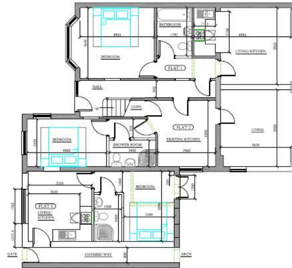
PROPOSED GROUND FLOOR PLAN SCALE 1:50
